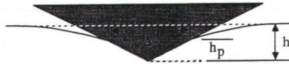
Fig. 94: Definition of the depths h and h_p used to determine the \gamma coefficient.
