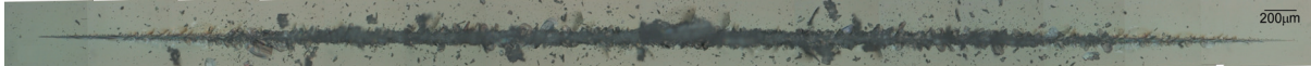
Fig. 74: Scratches (loading-unloading sequence with 3 N maximum) on a standard float glass and an annealed one.
