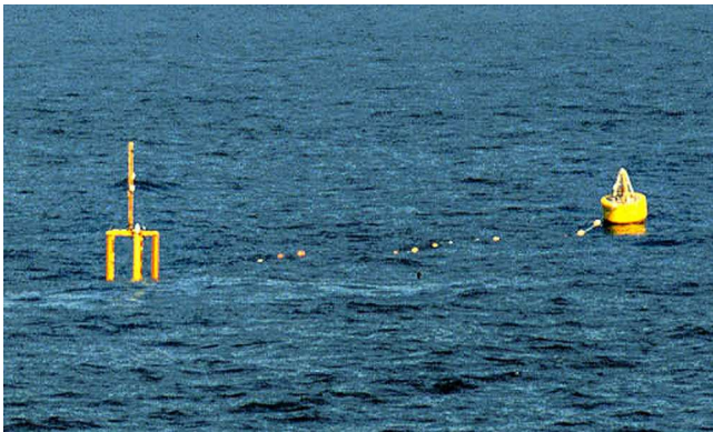
Figure 1: Photograph of the ASIS (left) and tether buoys deployed during FETCH. For scale, the mast on ASIS has a height of 4m.
