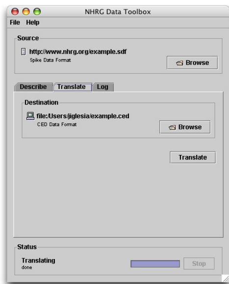
Figure 6.6: DataToolbox screenshot. The application is visually organized into 3 distinct parts. Top part defines the origin of the data to be manipulated (Source). Files and URLs can be dragged on the component. Alternatively, the “Browse” button can be hit to pop a file chooser up. Middle part is composed of tabs, one tab for each tool detected at start-up, plus one for the common “Log” tab. Each tool is responsible for laying down its front-end controls, help and output with unbound complexity. In the case of the “Translate” tool, it offers the possibility to choose a file (Destination) where data should be written to, along with the desired format, and a button to launch translation. The destination format is usually different from the source format. Bottom part shows a common “Status” bar providing information on what is going on in real time.
