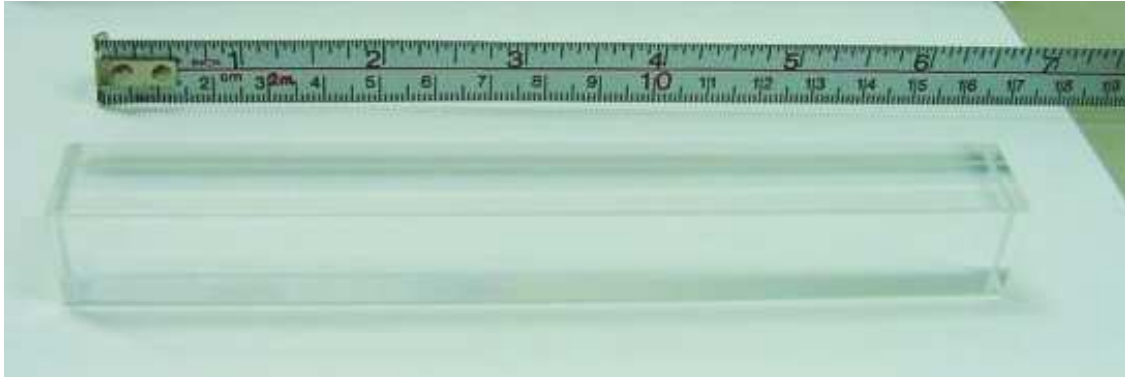
Figure 5.2: Single 150 mm long lead tungstate crystal picture as used for the laser-wire calorimeter.
