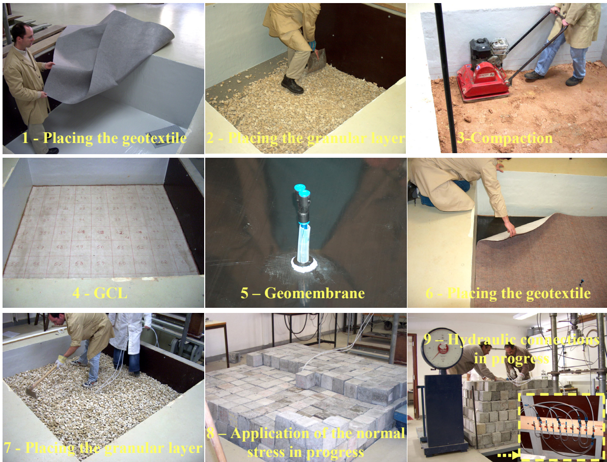
Figure 6.17 – Summary of large-scale test procedure
