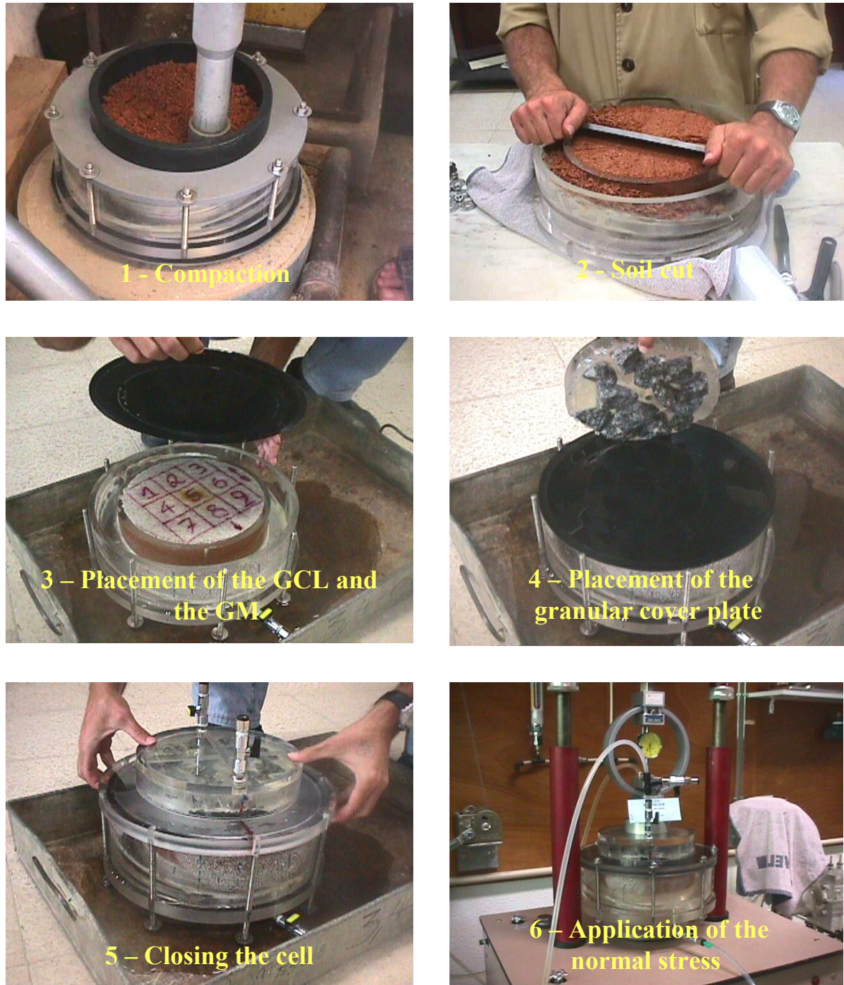
Figure 6.11 – Summary of small-scale test procedure
