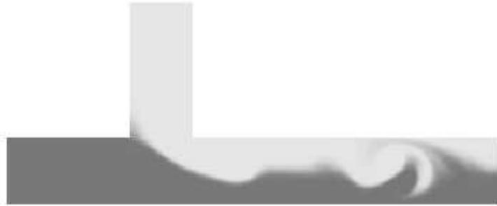
FIG. 4.3 – Instantaneous temperature fields in a 2D unsteady Tee junction at  $t = 12.2s$  (8 recirculation times) - non-physical temperature regions (*ie* out of limits) are denoted by dark contours.
