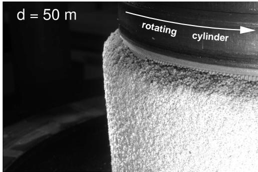
Fig. 5. Shear plane. When demounting the gouge sample after 50 m of slip, non-cohesive particles of the bulk are removed and an indurated plane is observed around the rotating cylinder. It consists of a crust made of weakly cemented particles.
