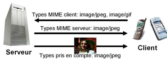
FIG. 2.1 – Principe des types MIME
