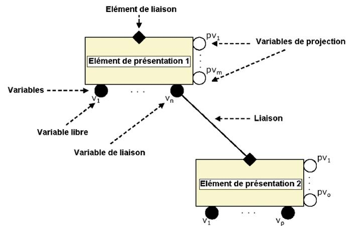
FIG. 2.19 – Éléments du modèle  $Z_YX$
