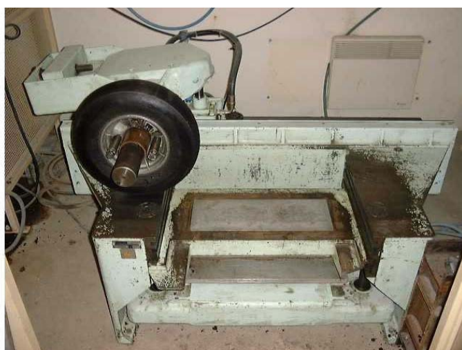
Figure II-3. Table de compactage LPC.
