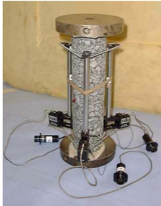
Figure III-12. Eprouvette type TSRST.
