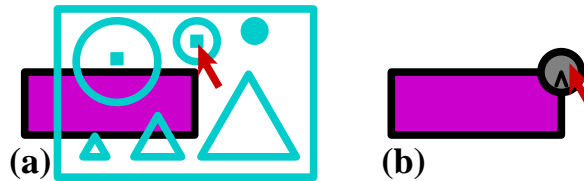
Figure 4.33: Creating and positioning objects with a Toolglass (adapted from Bier et al., 1993)
