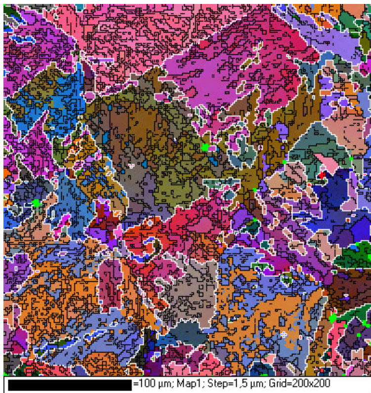
figure III. 5 : Cartographies EBSD. a) CGHAZ-100s, b) CGHAZ-500s
