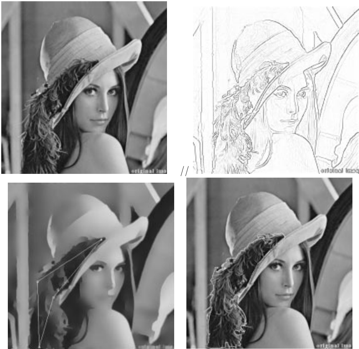
Fig. 7. Lena image. From top to bottom and left to right: the original image ( 512 \times 512 ), the Canny-Deriché gradient image ( \alpha = .35 ), the snake-spline initialization on the diffused image (100 iterations, \beta=6 \text{ E-}05 , s=5 and time to calculate equals 245 secondes), and the snake spline result with ( sp=3 , b=1 , sm=0 ).
