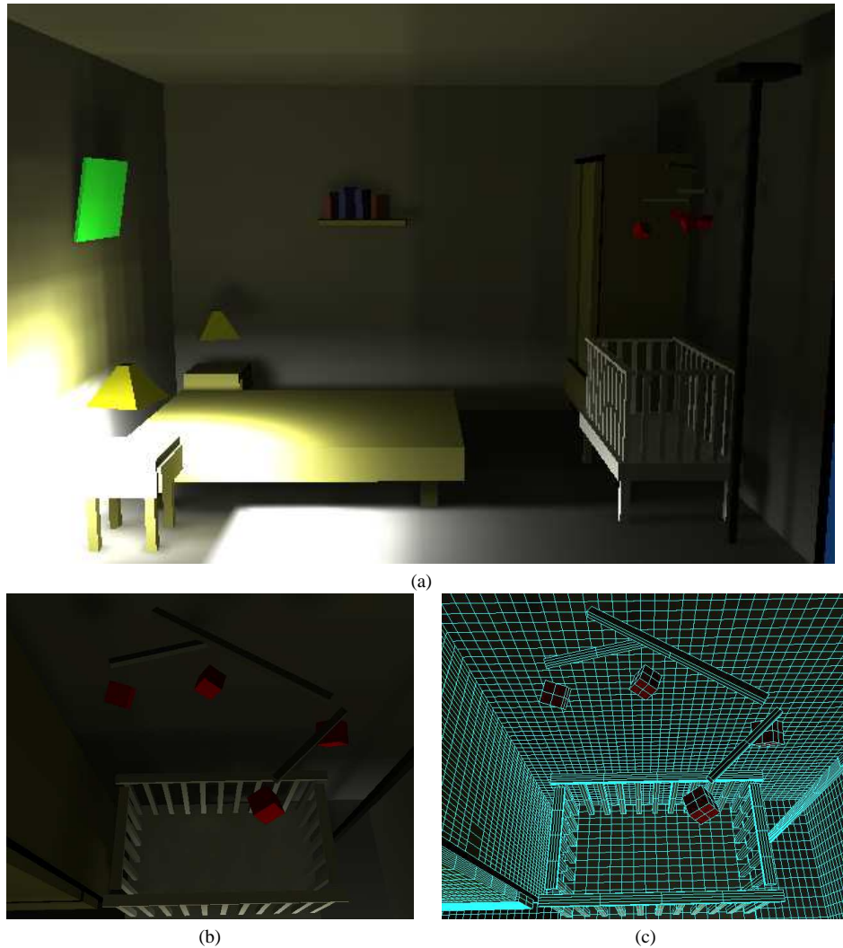
Fig. 27. Hierarchical Radiosity comparative results for Indirect Lighting scene: (a) the final image, (b) and (c) a closeup view of the right-hand wall.
