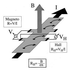
Figure 2.2: A typical Hall bar for measurement of the magnetoresitance R and the Hall resistance  $R_H$ . From [Sto99]
